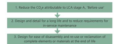
Design and detailing for a long life is achieved by following industry guidance on details and mix design appropriate to the service environment. If industry guidance is followed, the CO<sub>2</sub>e arising from requirements for structural maintenance during the design service life is usually minimal. Any benefits owing to the use of thermal mass to reduce heating or cooling needs are subject to assumptions about the rate of decarbonisation of the energy supply.
