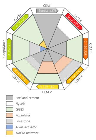
Fig 5.1: Typical carbon content of concretes made with different cements
