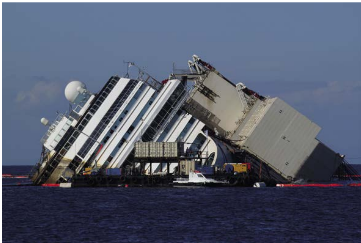
Parbuckling Concordia. (ph. credit Fagioli)
